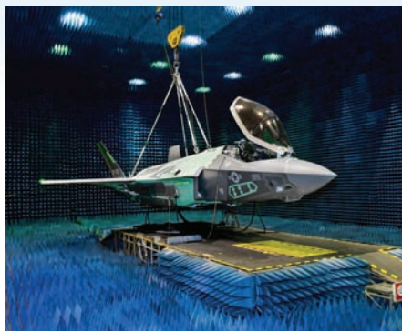
Anechoic chamber testing of the F-35A CTOL variant.
